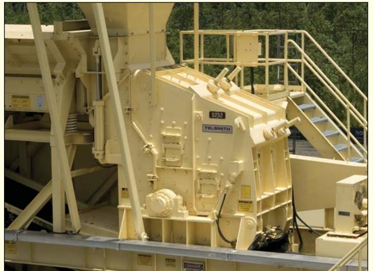
The RAP-fractionating or processing activity at P & S Paving begins with a front-end loader depositing RAP—the by-product of the company's road-milling operations—into the 42-in. x 16-ft. (1.0 x 4.9-m) TelSmith vibrating grizzly feeder (left photo, above). The material then passes to the TelSmith 5252
