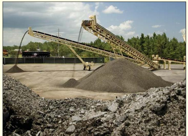
After leaving the Telsmith HSI crusher, the material moves to the PEP PSP 2618M screening plant (left photo, above). This unit has a double-deck high-frequency screen with a 6 x 18-ft. (1.8 x 5.5-m) top deck and a 6 x 12-ft. (1.8 x 3.7-m) bottom deck. The material is separated into two sizes, with oversize
