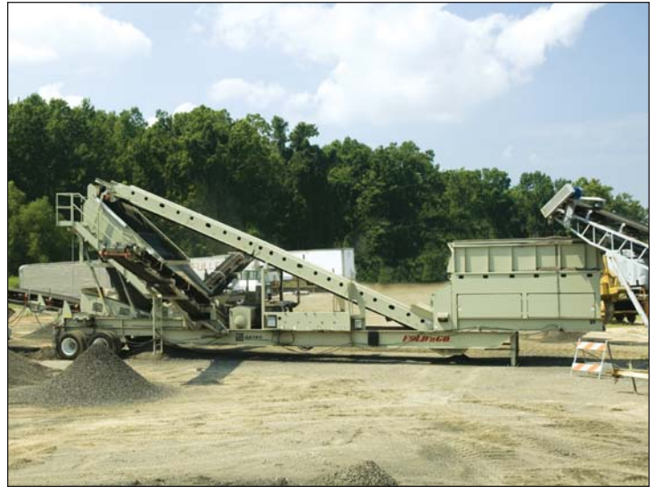
The management team at C.R. Jackson, Inc. made a quick decision to begin fractionating RAP as material costs climbed. They purchased this Astec Mobile Screens Fold 'n Go 2612V mobile screening plant (shown above in profile view) for the sole purpose of fractionating RAP.
