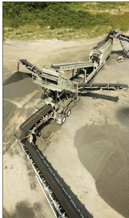
The management team at C.R. Jackson, Inc. made a quick decision to begin fractionating RAP as material costs climbed. They purchased this Astec Mobile Screens Fold 'n Go 2612V mobile screening plant (shown above in profile view) for the sole purpose of fractionating RAP.
