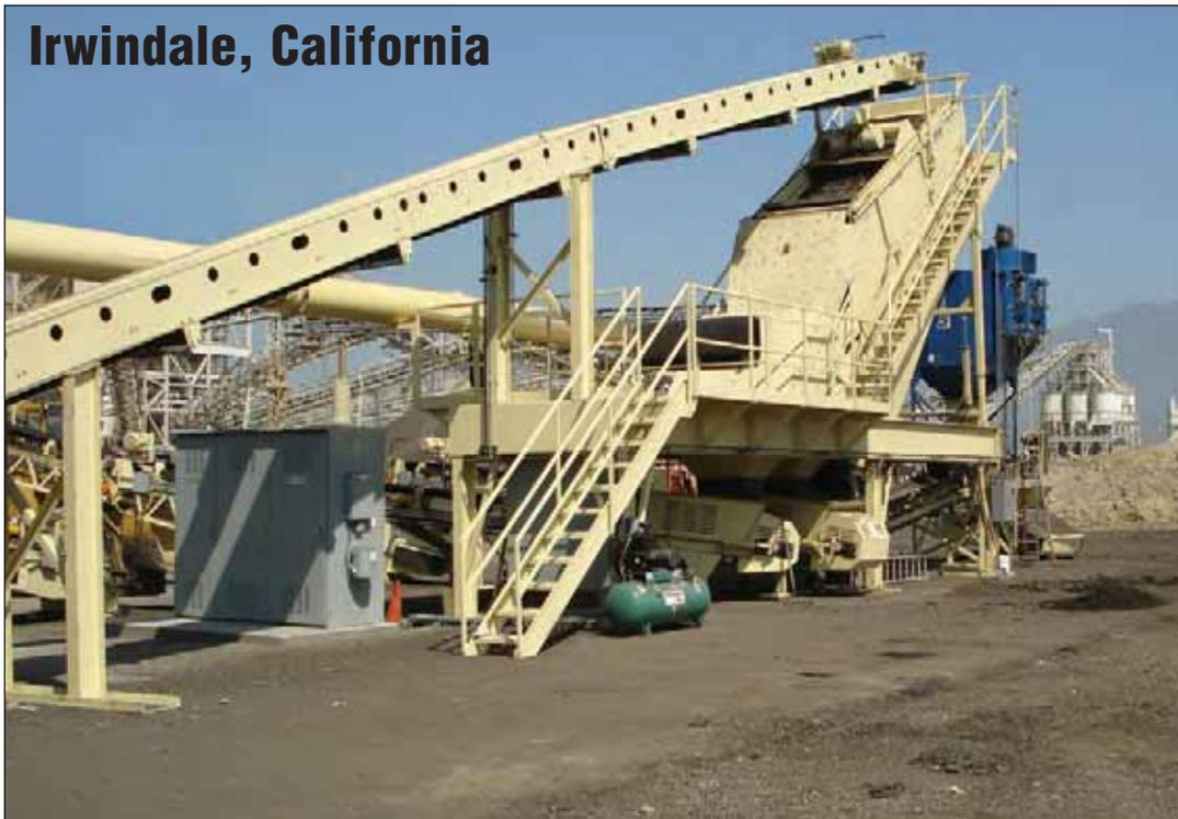
*The Irwindale, California facility is a stationary RAP-processing system equipped with a Telsmith 5252 HSI crusher and a 3618DM PEP screen. It also has two 80-ft. (24-m) stacking conveyors and a 100-ft. (30-m) radial stacker for returning the overs to the crusher for additional processing.*
