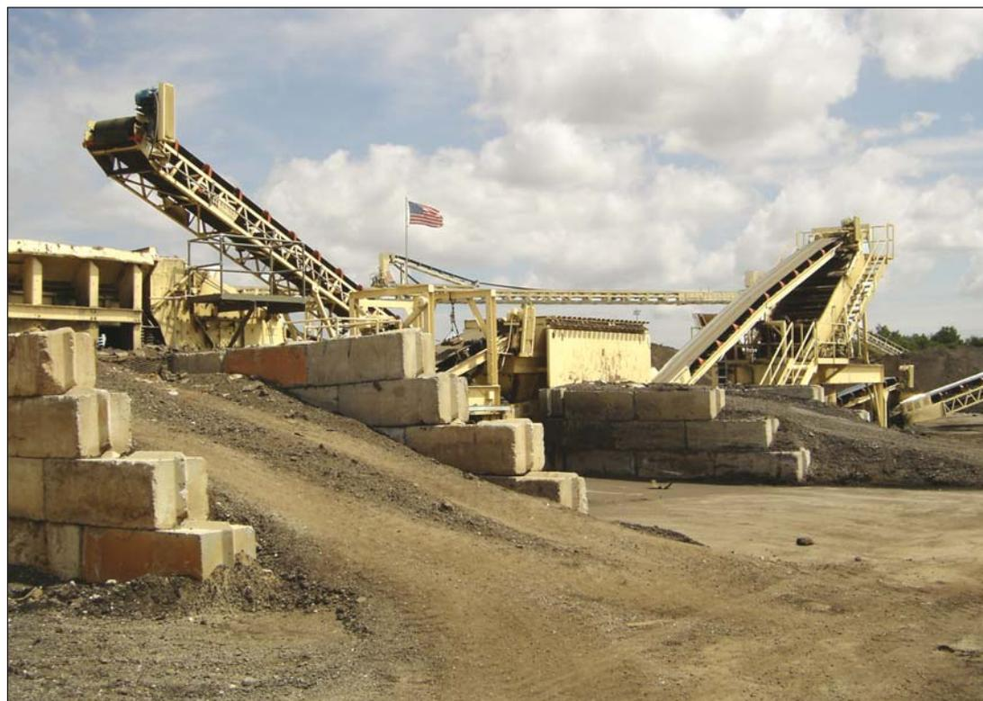
The STS 2618VM stationary screening plant from Astec Mobile Screens may be hard to spot in these photos of the Banks Construction Company plant site—but it is a key element in their effort to fractionate RAP to help them achieve high production rates while maintaining their tight quality-control standards. The STS 2618VM screens the RAP material into two sizes. The company maintains stockpiles of about 4,000 tons (3,600 tonnes) of each size of RAP.
